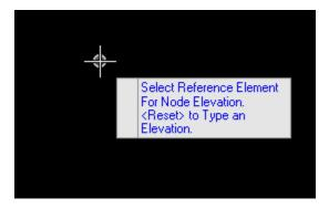
For this example, use 1172.450, the invert flowline elevation of the design structure. Then, hit the enter key and it will lock this elevation.
