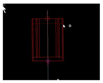
Repeat this on the other end and/or at any vertices along the conduit using the appropriate node in each location.
