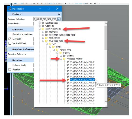
Then select the feature of the node to be placed. For this example, place a P 06 x 03 CIP SGL PW 0
