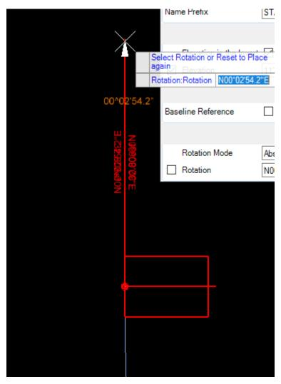
Snap to the ASCII graphics to set the rotation to the PRO graphic from the ASCII input. Then data point to accept.
