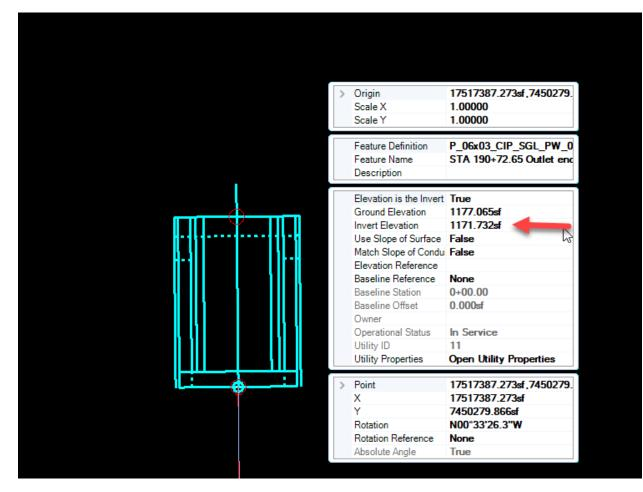
This will correct the elevation placement.
